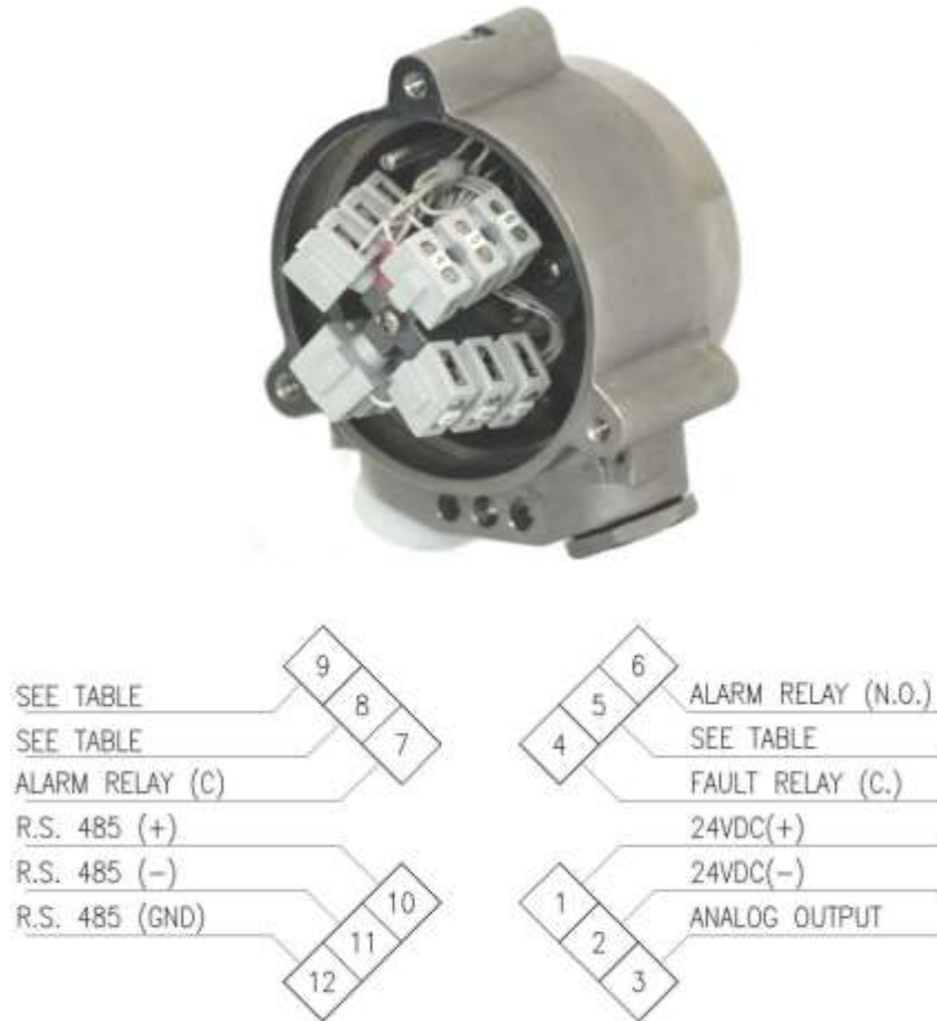
Figure 8: Wiring Terminals
