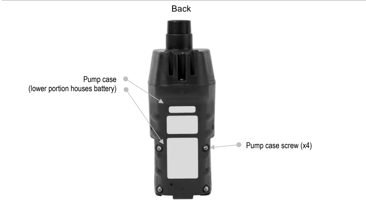
Figure 3.1.B Hardware overview aspirated instrument
