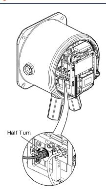
Ensure the pneumatic tubes are properly identified for later connection to the correct connectors.
