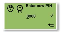
On the "Enter new PIN" screen, use Switch 2 to cycle through the values to set the first digit. Use Switch 1 to move to the next digit.
