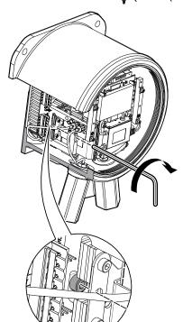
If the module is in its correct position, the screws will engage in the threads and turn freely.
