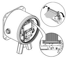
Press the 'wings' down to release the ribbon cable at the top of the Detection Module.
