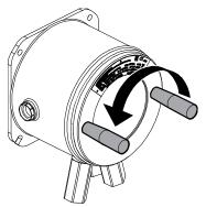
Turn counter-clockwise to unscrew the front cover.
