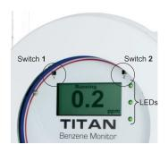
LEDs Green Titan is operating correctly.
