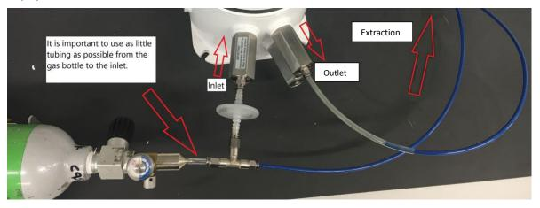
If the Titan does not display the gas concentration given by the bottle, calibrate the Titan to give the correct readings. Refer to:
