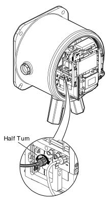
Check the identification of the pneumatic tubes and connectors.
