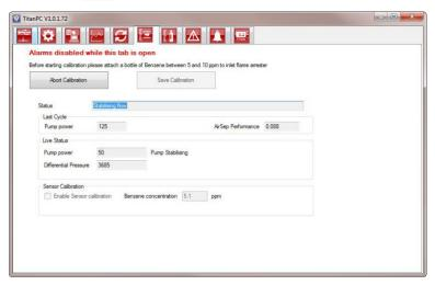
Attach a bottle of between 5 and 10ppm Benzene to the inlet flame-arrestor before you start calibration. This ensures the benzene is flowing through the Titan system before the start of the calibration.
