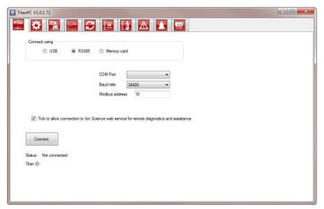
Click on the radio button for USB or RS485, to select the connection type.
